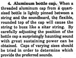
NOTE: any plastic gaskets that are attached to the cap should be removed in order to allow the cap to vibrate freely.
